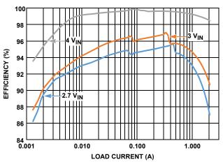
FIGURE 2. EFFICIENCY vs LOAD CURRENT,  $V_{OUT} = 3.3V$
