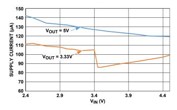
FIGURE 7. SUPPLY CURRENT vs  $V_{\mbox{\scriptsize IN}}$
