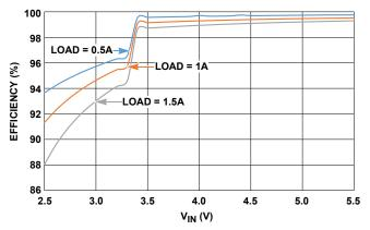
FIGURE 4. EFFICIENCY vs  $V_{IN}$ ,  $V_{OUT} = 3.3V$
