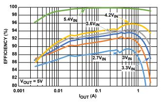
FIGURE 6. EFFICIENCY vs LOAD CURRENT,  $V_{OUT} = 5V$
