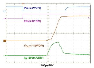
FIGURE 10. START-UP WAVEFORM  $50\Omega$  LOAD,  $V_{\text{IN}}$  = 3V,  $V_{\text{OUT}}$  = 3.3V
