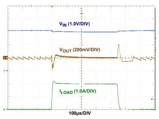
FIGURE 12. LOAD STEP RESPONSE,  $V_{IN} = 3V$ ,  $I_{OUT} = 10mA -> 1500mA -> 10mA$
