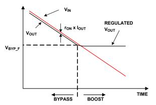
FIGURE 18. AUTO BYPASS WITH FALLING VIN
