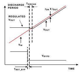
FIGURE 21. FORCED MODE, BOOST TO BYPASS
