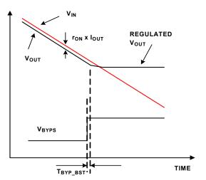
FIGURE 20. FORCED MODE, BYPASS TO BOOST
