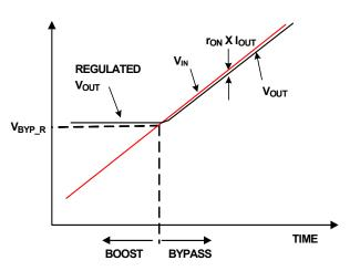
FIGURE 19. AUTO BYPASS WITH RISING  $V_{\mbox{\scriptsize IN}}$
