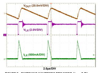
FIGURE 8. SWITCHING WAVEFORM PFM MODE,  $V_{\mbox{\footnotesize{IN}}}$  = 2.7V,  $I_{\mbox{\footnotesize{LOAD}}}$  = 50  $\Omega,~V_{\mbox{\footnotesize{OUT}}}$  = 3.3V
