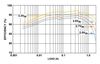
FIGURE 5. EFFICIENCY vs LOAD CURRENT, V<sub>OUT</sub> = 3.5V
