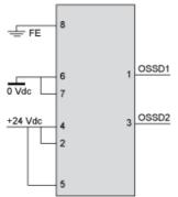
With External Device Monitoring (EDM) feedback loop
