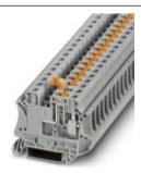
Knife disconnect terminal block, Connection type: Screw connection, Cross section: 0.2 mm² - 10 mm², AWG: 24 - 8, Nominal current: 20 A, Nominal voltage: 500 V, Length: 57.8 mm, Width: 8.2 mm, Color: blue, Assembly: NS 35/7,5, NS 35/15
