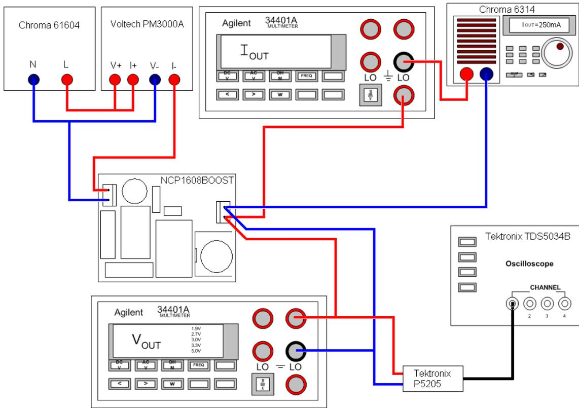
Figure 36. Test Setup
