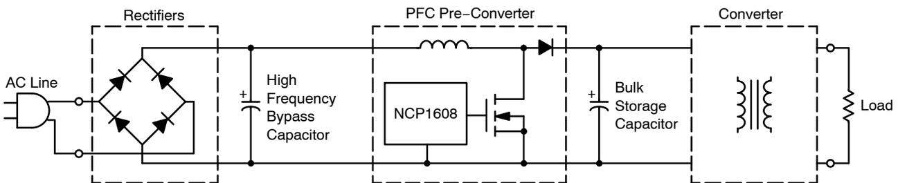
Figure 1. Active PFC Stage with the NCP1608
