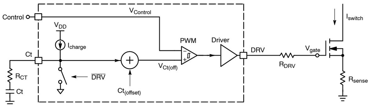
Figure 18. Block Diagram of the Propagation Delay Components
