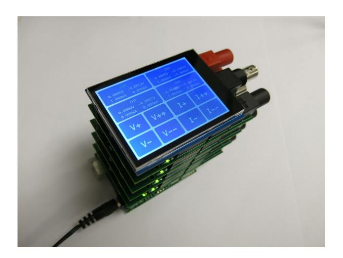
It is recommended to set the Linduino JP3 jumper to the EXT position when using the EasySMU shield. The QuikEval $^{\text{TM}}$  connector is not used by the EasySMU, so
