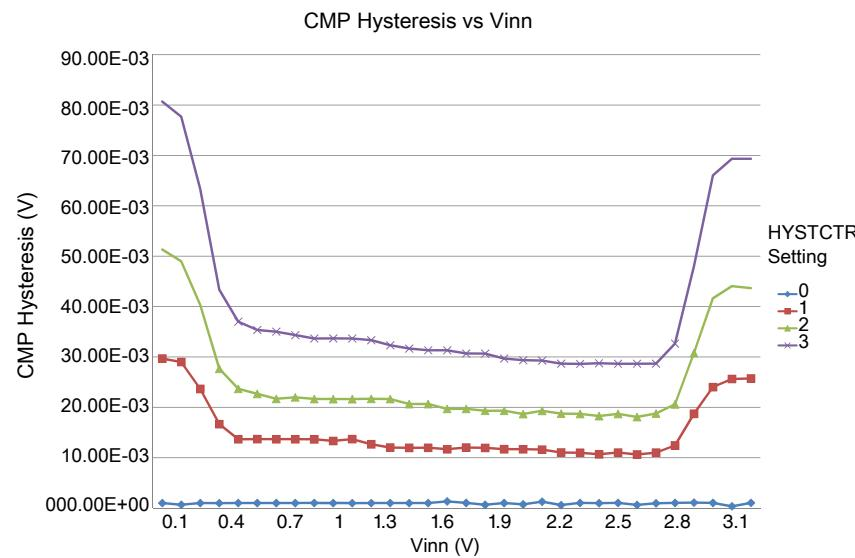
**Figure 10. Typical hysteresis vs. Vin level (V<sub>DD</sub> = 3.3 V, PMODE = 0)**
