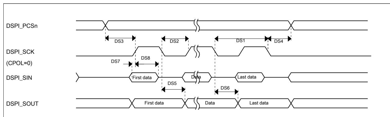
**Figure 14. DSPI classic SPI timing — master mode**
