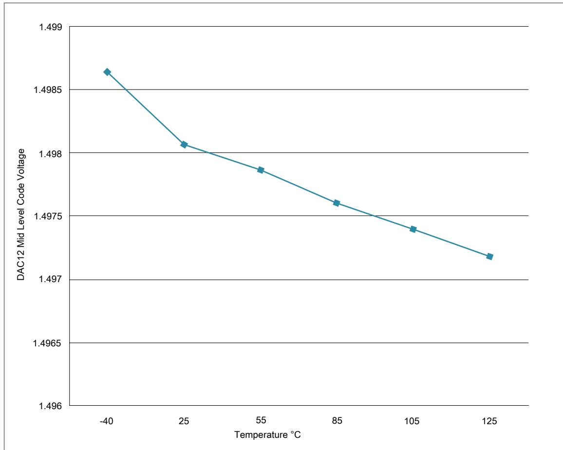
**Figure 13. Offset at half scale vs. temperature**
