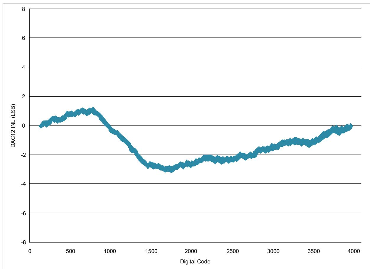
**Figure 12. Typical INL error vs. digital code**
