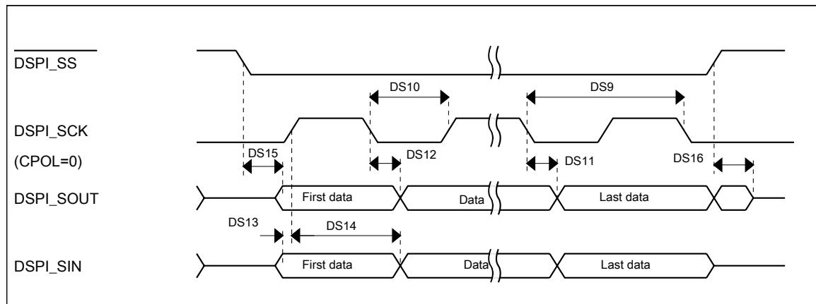
**Figure 17. DSPI classic SPI timing — slave mode**
