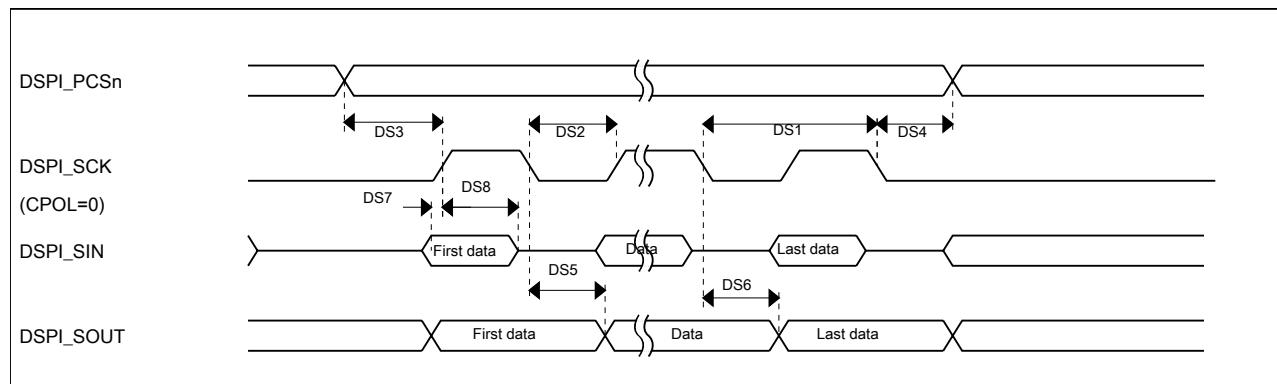
**Figure 16. DSPI classic SPI timing — master mode****Table 29. Slave mode DSPI timing (full voltage range)**
