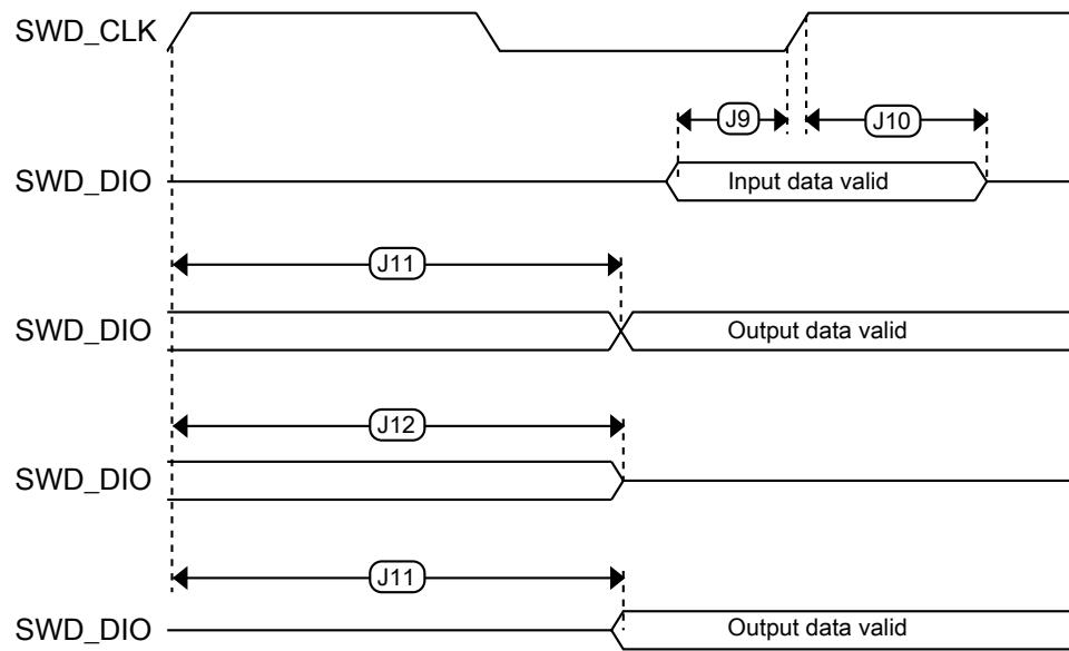
**Figure 6. Serial wire data timing**
