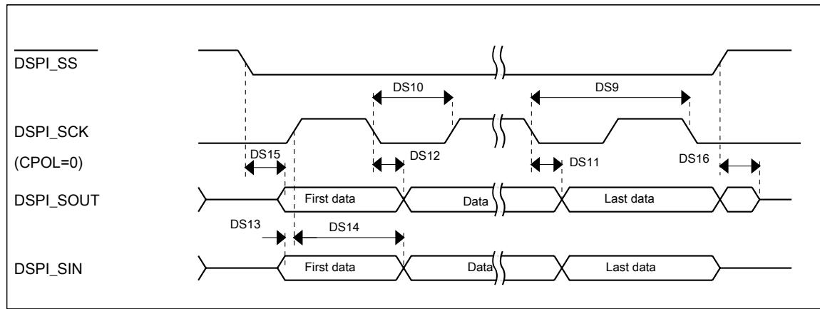
**Figure 15. DSPI classic SPI timing — slave mode**
