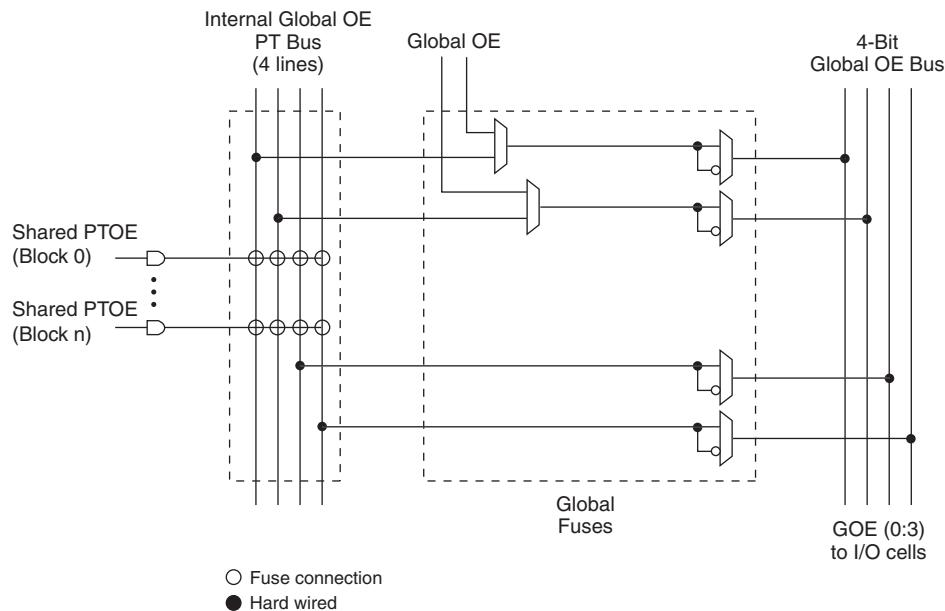
**Figure 10. Global OE Generation for ispMACH 4032**
