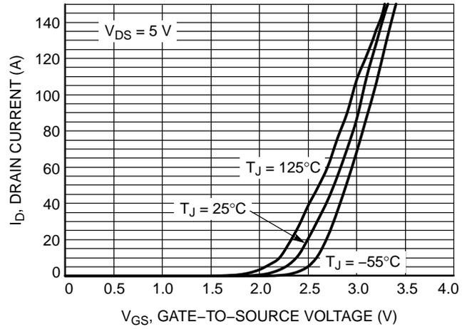
Figure 2. Transfer Characteristics
