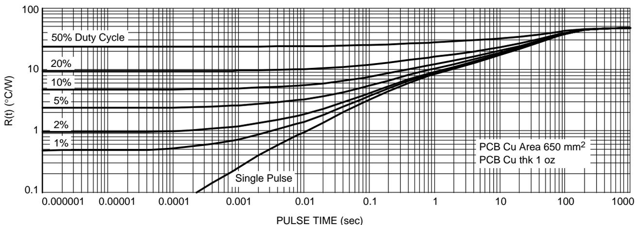
Figure 13. Thermal Characteristics
