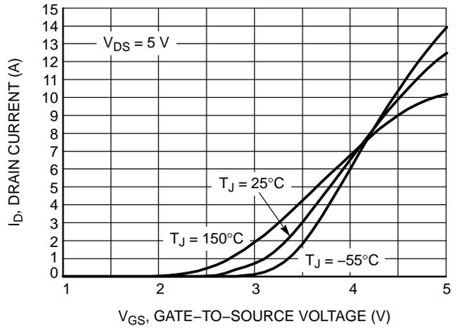
Figure 2. Transfer Characteristics
