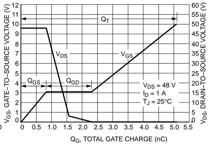
Figure 10. Gate-to-Source and Drain-to-Source Voltage vs. Total Charge
