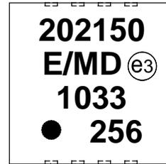
8-Lead DFN-S (6x5x0.9 mm)
