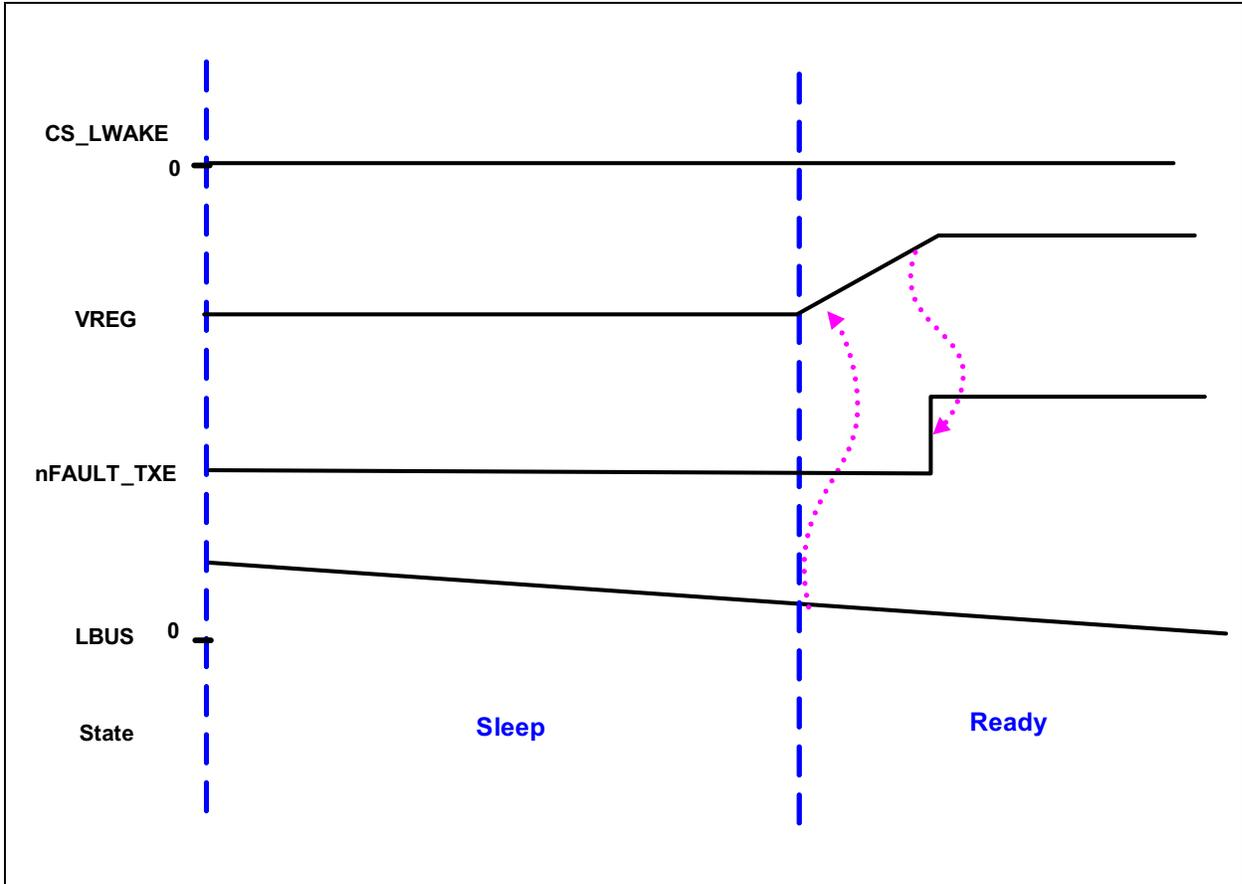
**FIGURE 1-4:** MCP2021P/2P Wake-Up Due to Bus Disconnecting.
