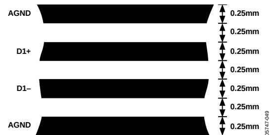
Figure 61. Arrangement of Signal Tracks
