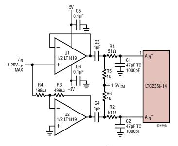
Figure 6a. The LT1819 Driving the LTC2356-14 Differentially
