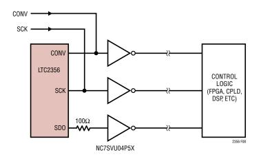
Figure 8. Serial Interface with Buffers
