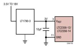
Figure 3. Overdriving V<sub>REF</sub> Pin with an External Reference
