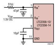
Figure 1. RC Input Filter
