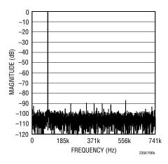
Figure 6b. LTC2356-12 6MHz Sine Wave 4096 Point FFT Plot with the LT1819 Driving the Inputs Differentially
