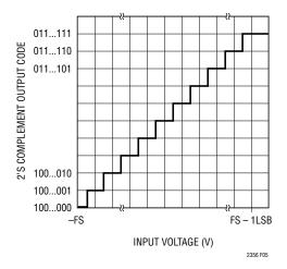
Figure 5. LTC2356-12/LTC2356-14 Transfer Characteristic
