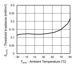
Fig. 9 - Sensitivity vs. Ambient Temperature
