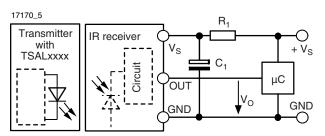
$\rm R_1$  and  $\rm C_1$  are recommended for protection against EOS. Components should be in the range of 33  $\Omega$  <  $\rm R_1$  < 1 k $\Omega$ ,  $\rm C_1$  > 0.1  $\mu F$ .
