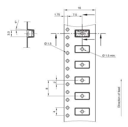
technical drawings according to DIN specifications
