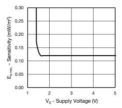
Fig. 12 - Sensitivity vs. Supply Voltage
