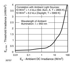
Fig. 6 - Sensitivity in Bright Ambient
