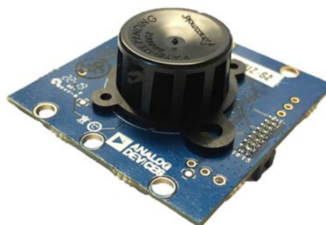
Figure 46. EVAL-CHAMBER Smoke Chamber
