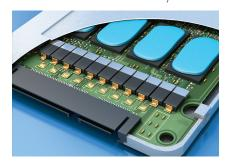
Gap Filler 4000 is a two-part, high performance, thermally conductive, liquid gap filling material. The mixed material will cure at room temperature and can be accelerated with the addition of heat. Gap Filler 4000 offers an extended working time to allow greater flexibility in the customer's assembly process.
