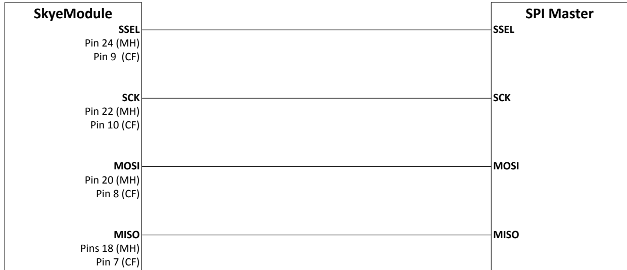
Figure 9-3: SPI Connection Diagram
