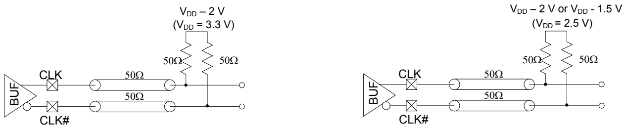
Figure 15. LVPECL Termination
