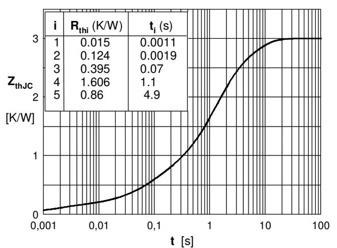
Fig. 8 Transient thermal impedance junction to case
