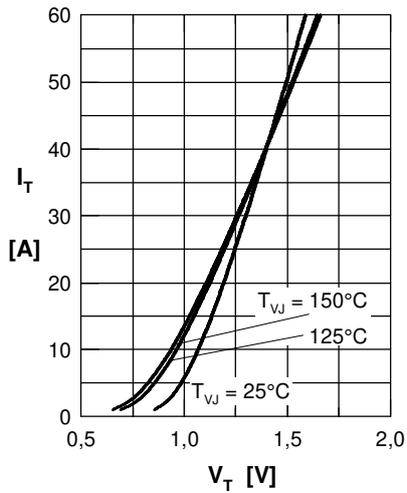
Fig. 1 Forward characteristics
