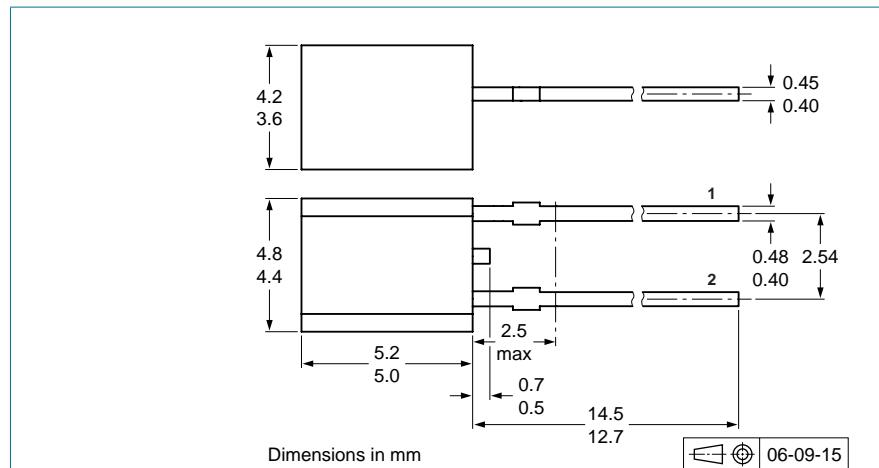
Fig 4. Minimized package outline SOD70
