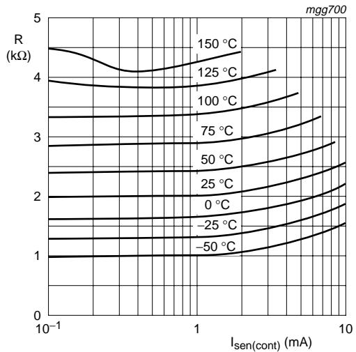
To keep the temperature error low, an operating current of  $I_{\text{sen(cont)}} = 1 \text{ mA}$  is recommended for temperatures above 100 °C
