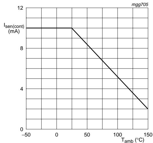
Fig 3. Maximum operating current for safe operation
