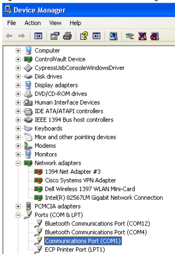
Figure 8-22. Serial Ports List in Device Manager Window
