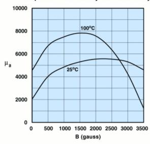
Measured on an 18/10/6mm toroid at 10kHz.
