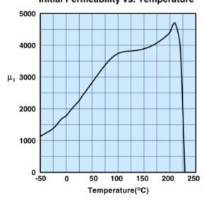
Measured on an 18/10/6mm toroid at 100kHz.
