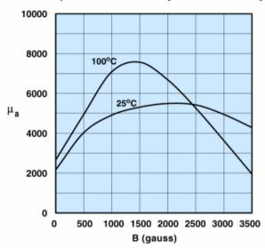
Measured on an 18/10/6mm toroid at 10kHz.
