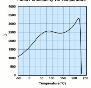
Measured on an 18/10/6mm toroid at 100kHz.
