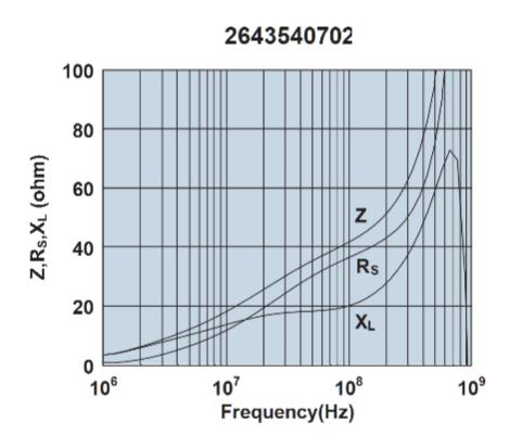
Impedance, reactance, and resistance vs. frequency.
