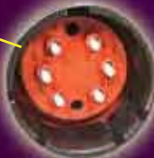
ARINC 801 Fiber Optic Connector and Termini
