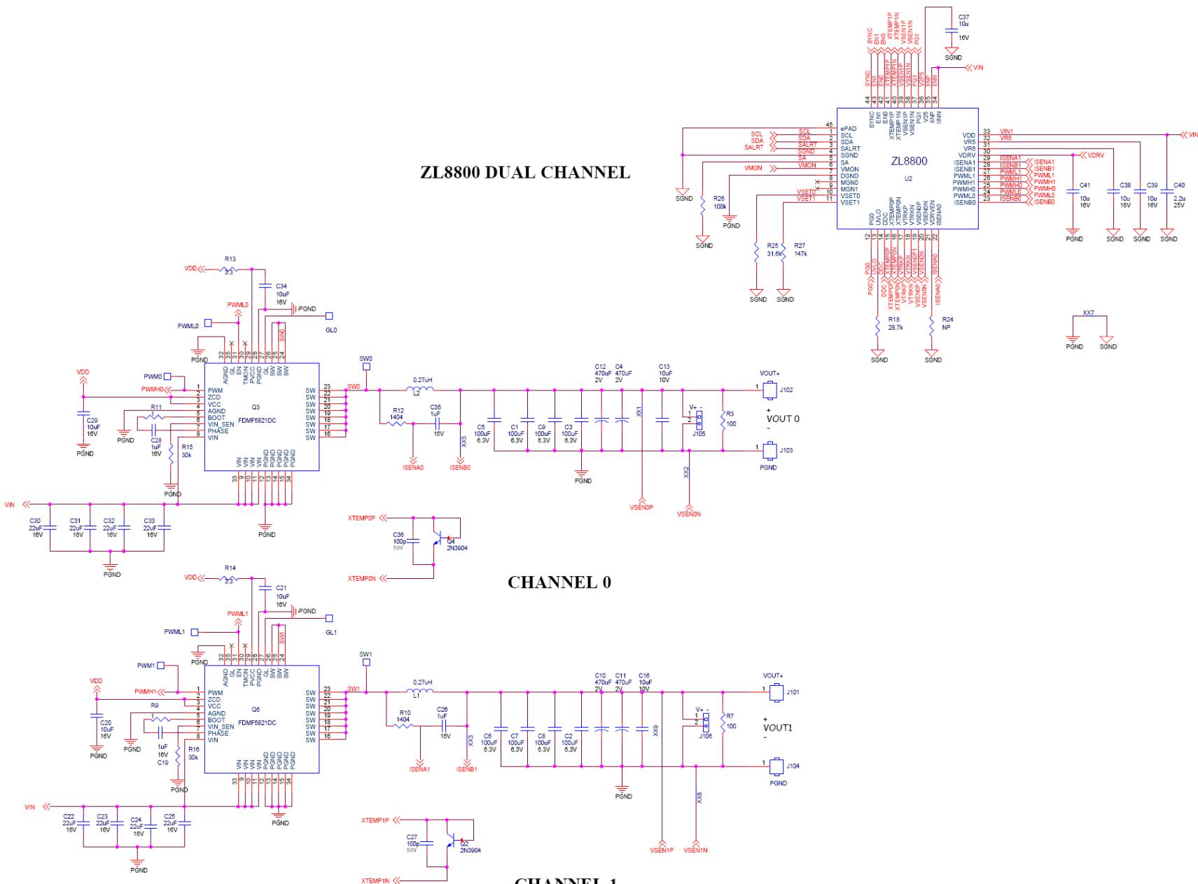
FIGURE 2. APPLICATION CIRCUIT
