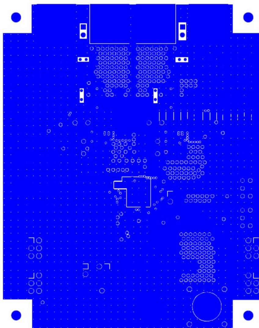
**FIGURE 17. PCB - INNER LAYER 1 (TOP VIEW)**
