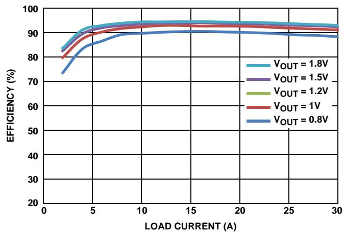
FIGURE 8. EFFICIENCY,  $V_{IN} = 5V$ ,  $f_{SW} = 400kHz$
