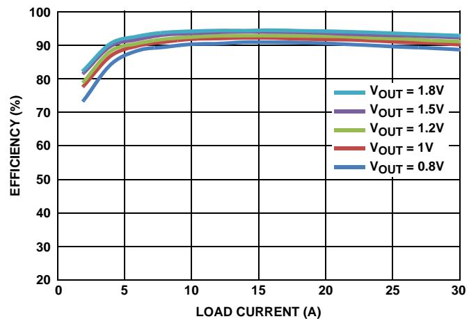
FIGURE 6. EFFICIENCY,  $V_{IN} = 5V$ ,  $f_{SW} = 300kHz$
