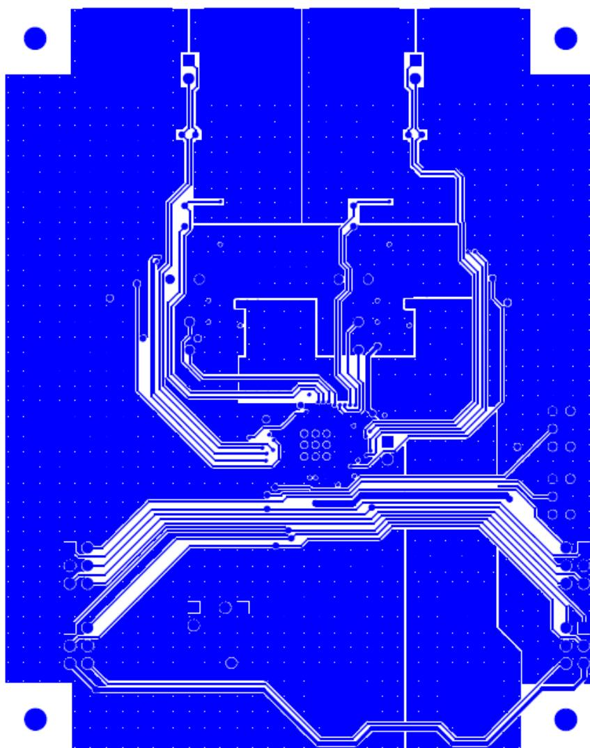
**FIGURE 18. PCB - INNER LAYER 2 (TOP VIEW)**
