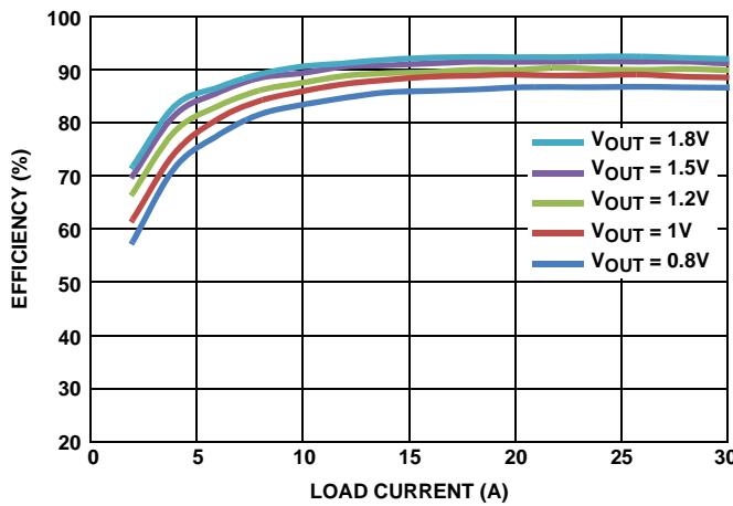
FIGURE 7. EFFICIENCY,  $V_{IN} = 12V$ ,  $f_{SW} = 400kHz$
