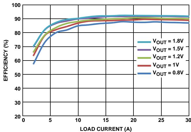
FIGURE 5. EFFICIENCY,  $V_{IN} = 12V$ ,  $f_{SW} = 300kHz$
