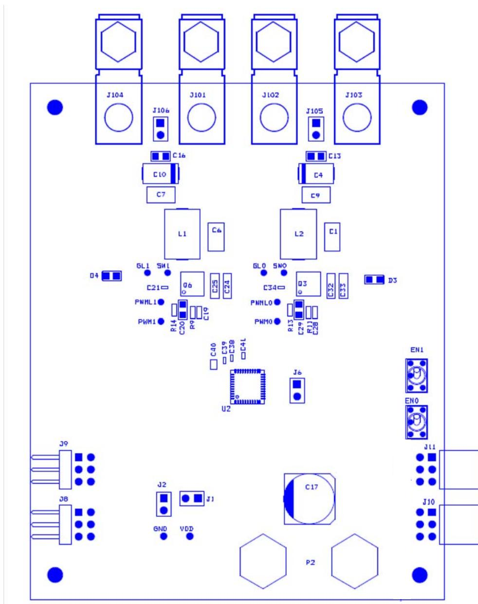
**FIGURE 15. PCB - TOP ASSEMBLY**
