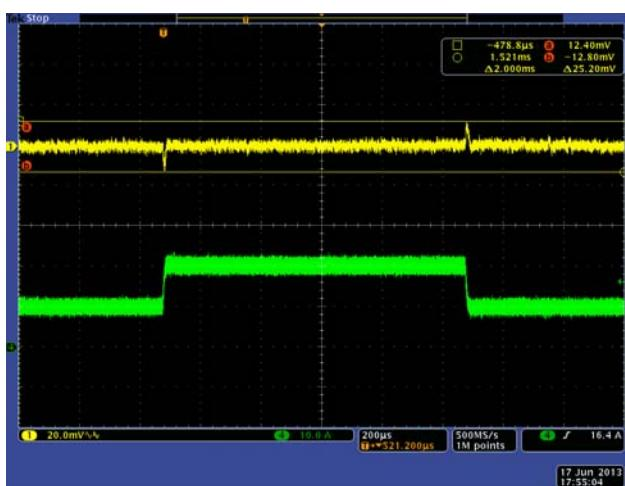
FIGURE 13. STEP RESPONSE, 10A TO 20A @ 5A/μs, ASCR = 1000
