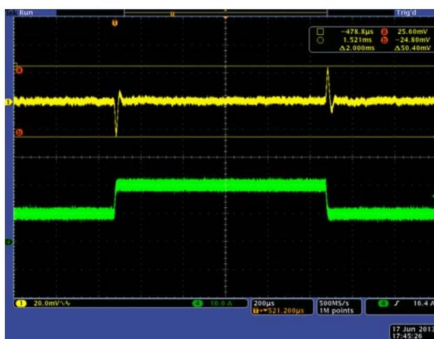
FIGURE 14. STEP RESPONSE, 10A TO 20A @ 5A/μs, ASCR = 400
