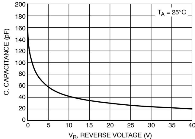
Figure 3. Typical Capacitance
