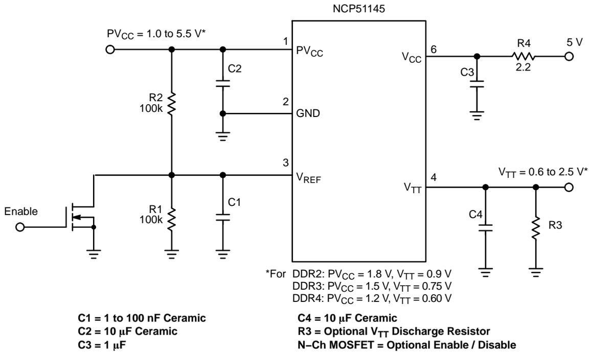
Figure 1. Application Diagram
