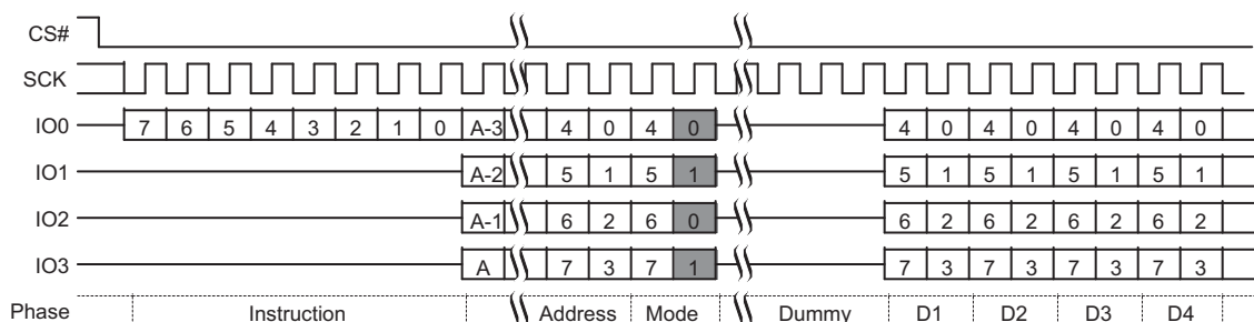
Figure 80. Quad I/O Read Command Sequence (EBh or ECh)
