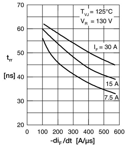
Fig. 5 Typ. recov. time  $t_{rr}$  versus  $-di_F/dt$
