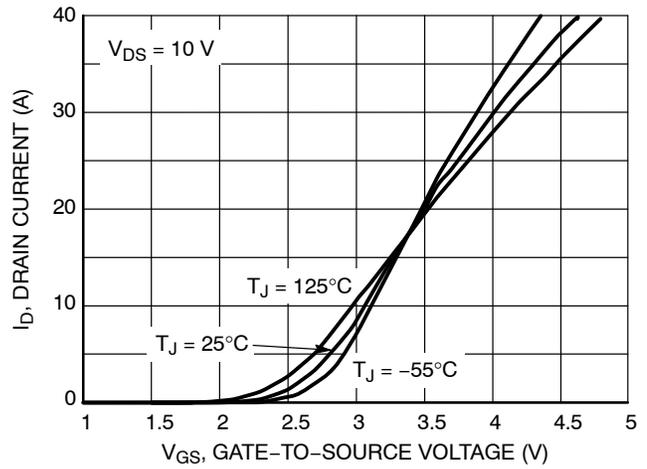
Figure 2. Transfer Characteristics
