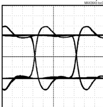
ELECTRICAL EYE DIAGRAM (2.5Gbps, I_{MOD} = 30mA , PATTERN = PRBS 2^7 - 1 + 80 CID)
