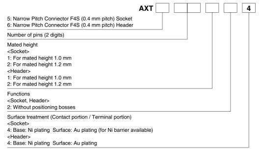
Note: Please note that models with a mated height of 1.0 mm (7th digit of part number is "1") and 1.2 mm (7th digit of part number is "2") are not compatible.
