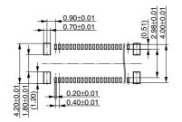
Recommended metal mask opening pattern Metal mask thickness: When 120µm (Terminal opening ratio: 60%) (Metal-part opening ratio: 100%)
