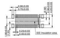
Recommended metal mask opening pattern Metal mask thickness: When 150µm (Terminal opening ratio: 48%) (Metal-part opening ratio: 100%)
