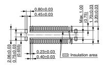
Recommended metal mask opening pattern Metal mask thickness: When 150µm (Terminal opening ratio: 48%)
