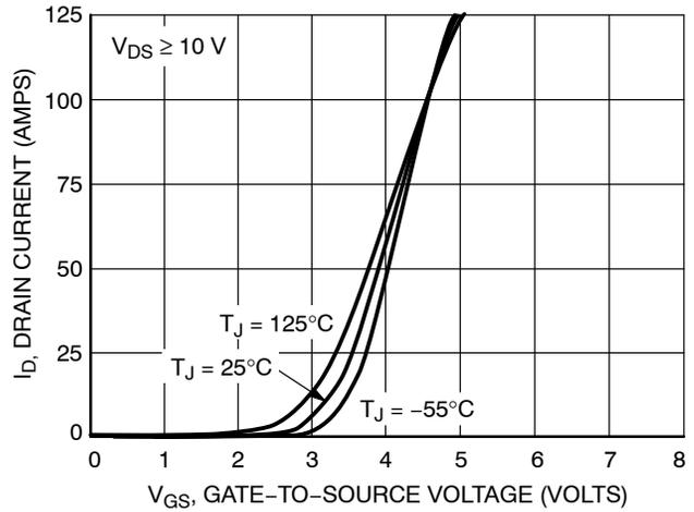
Figure 2. Transfer Characteristics
