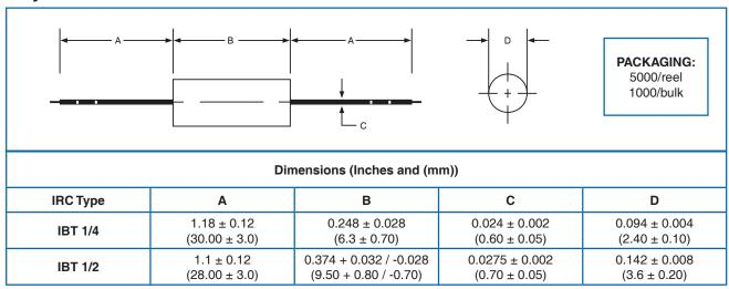
Application notes - Lead forming within 2mm of the body and soldering within 4mm of the body are not recommended. Owing to the hydroscopic nature of carbon composition technology, aqueous washing is not recommended.
