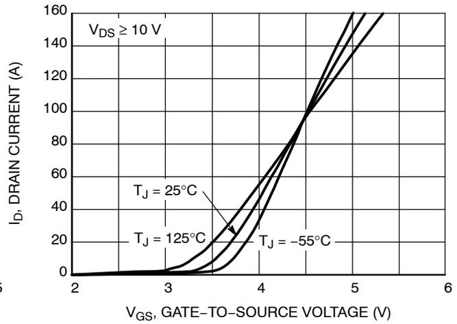
Figure 2. Transfer Characteristics
