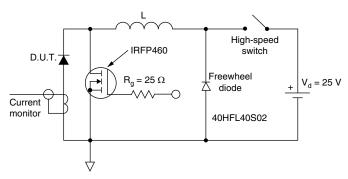
Fig. 8 - Unclamped Inductive Test Circuit
