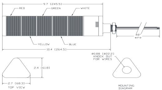
LED OPERATION: CONNECT STACK COLOR WIRE TO POWER AND BROWN WIRE TO POWER.
