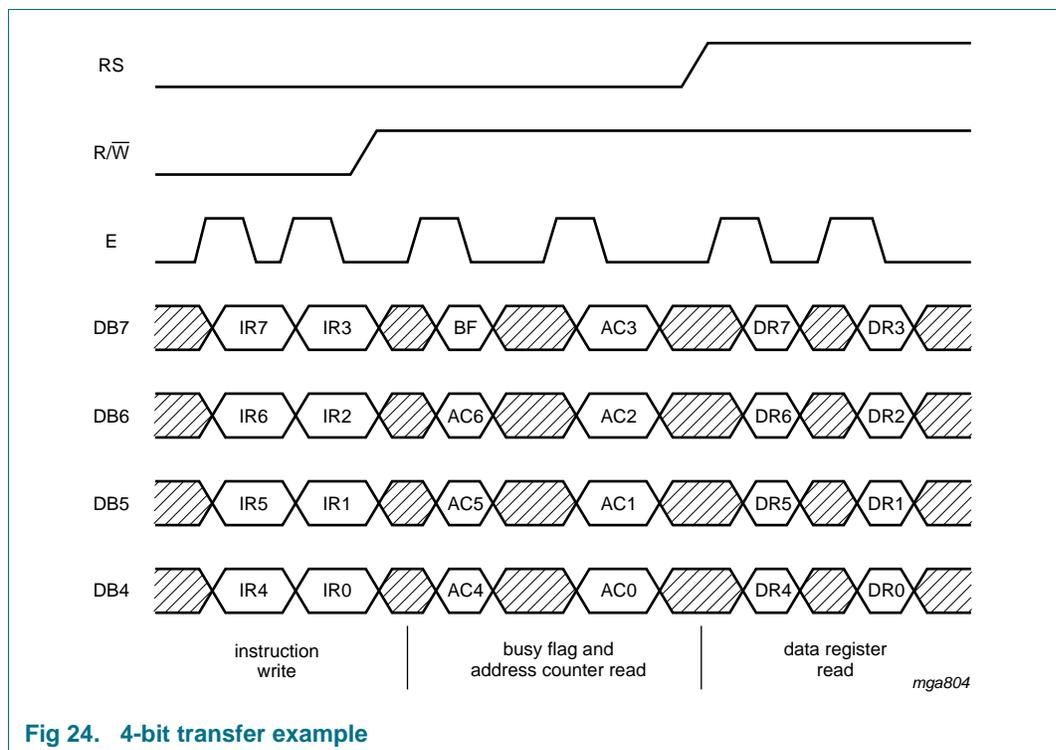
**Fig 24. 4-bit transfer example**
