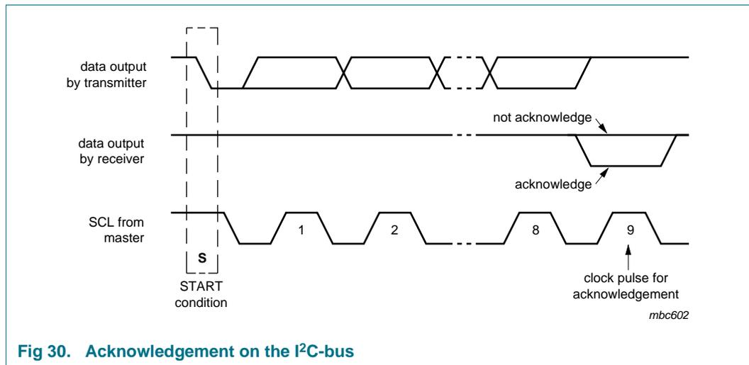
Fig 30. Acknowledgement on the I<sup>2</sup>C-bus
