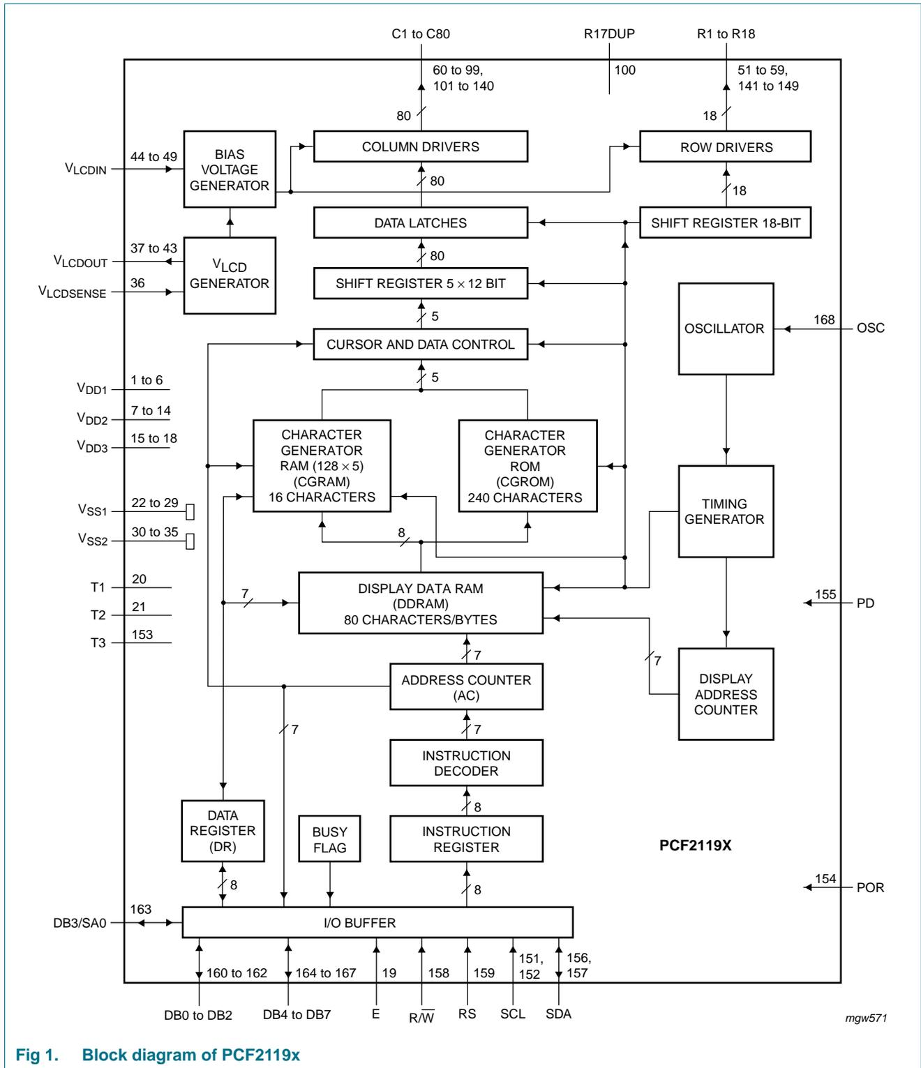
Fig 1. Block diagram of PCF2119x
