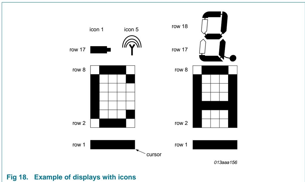
**Fig 18. Example of displays with icons**
