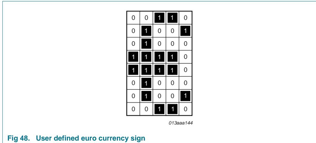
Below some source code is printed, which shows how a user defined character is defined - in this case the euro currency sign. The display used is a 2 lines by 16 characters display and the interface is the I<sup>2</sup>C-bus:
