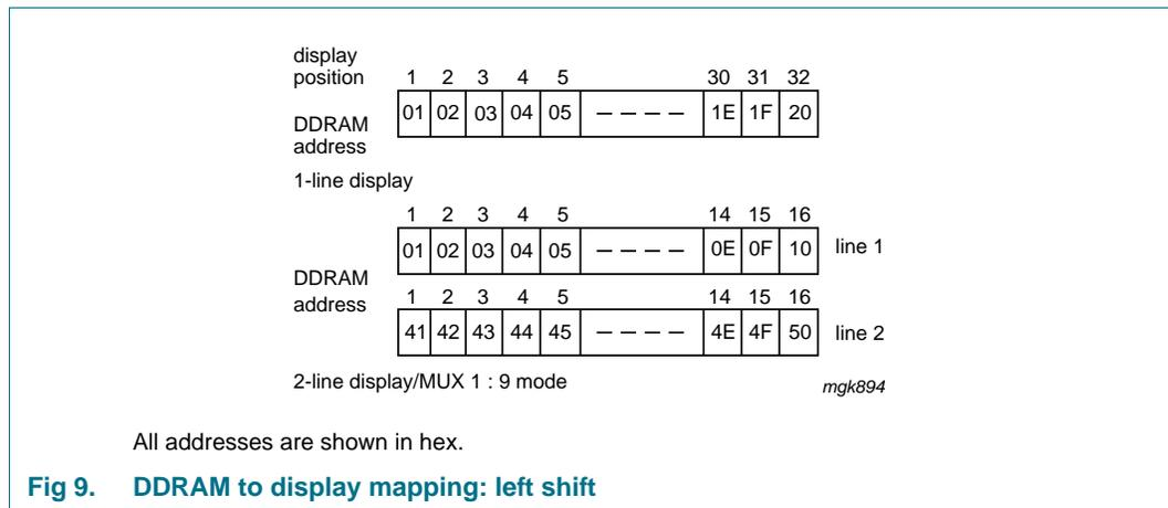
When data is written to or read from the DDRAM, wrap-around occurs from the end of one line to the start of the next line. When the display is shifted each line wraps around within itself, independently of the others. Thus all lines are shifted and wrapped around together. The address ranges and wrap-around operations for the various modes are shown in [Table 7](#).
