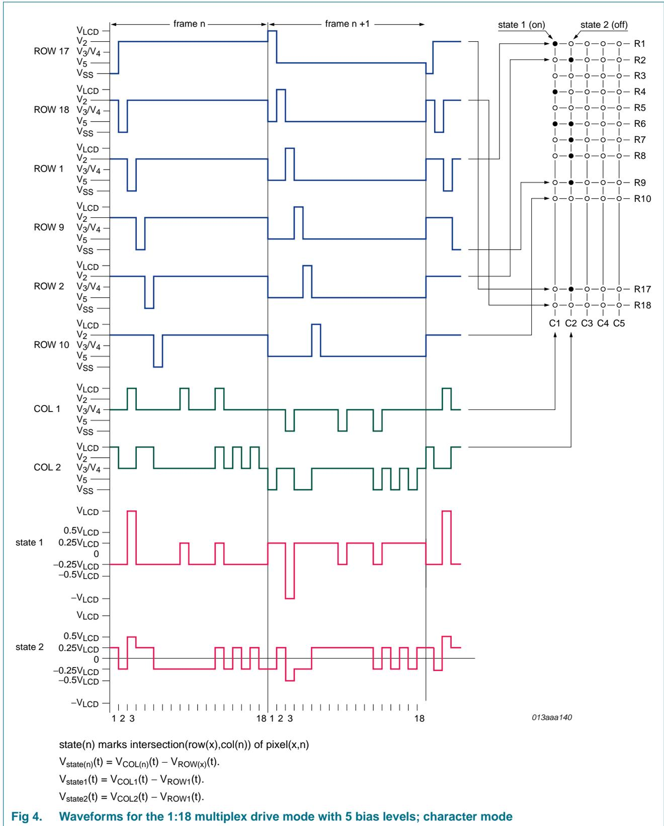
**Fig 4. Waveforms for the 1:18 multiplex drive mode with 5 bias levels; character mode**
