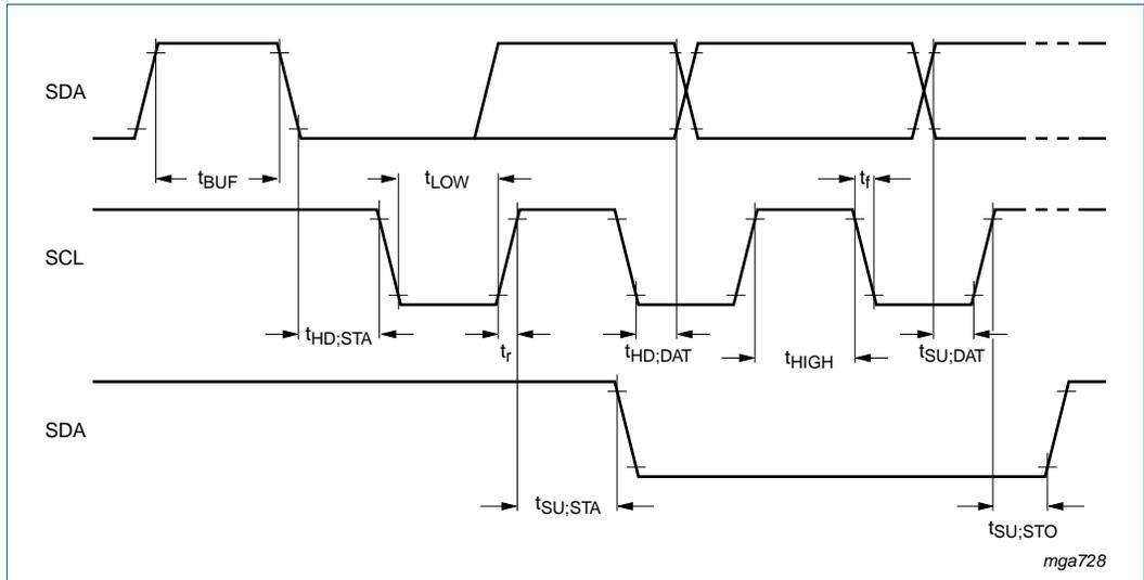
Fig 36. I<sup>2</sup>C-bus timing diagram
