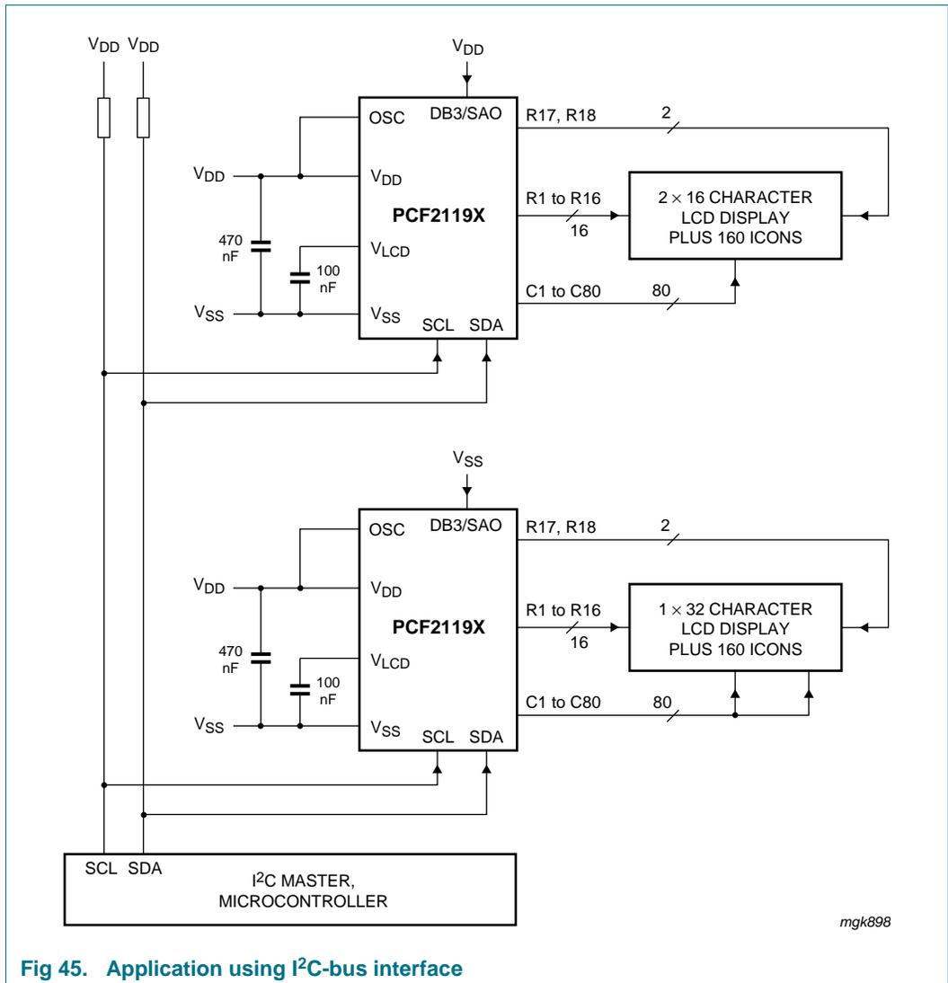
Fig 45. Application using I<sup>2</sup>C-bus interface
