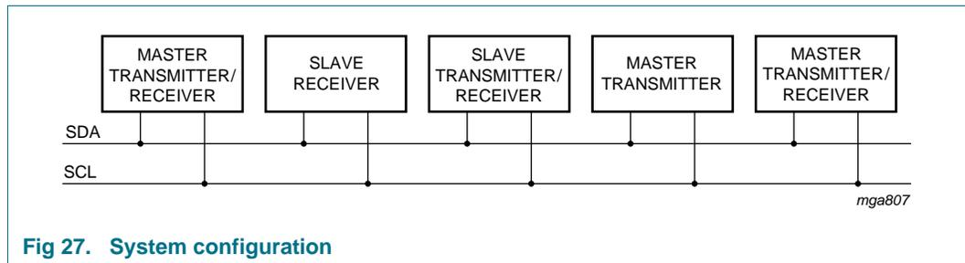
Fig 27. System configuration
