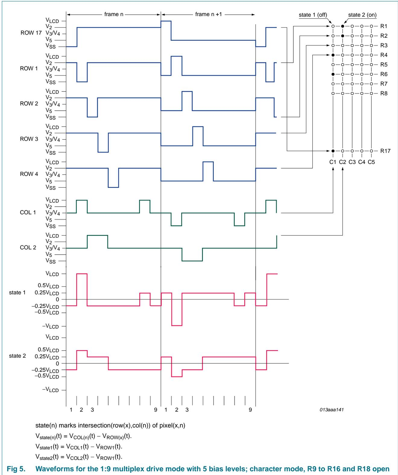
**Fig 5. Waveforms for the 1:9 multiplex drive mode with 5 bias levels; character mode, R9 to R16 and R18 open**
