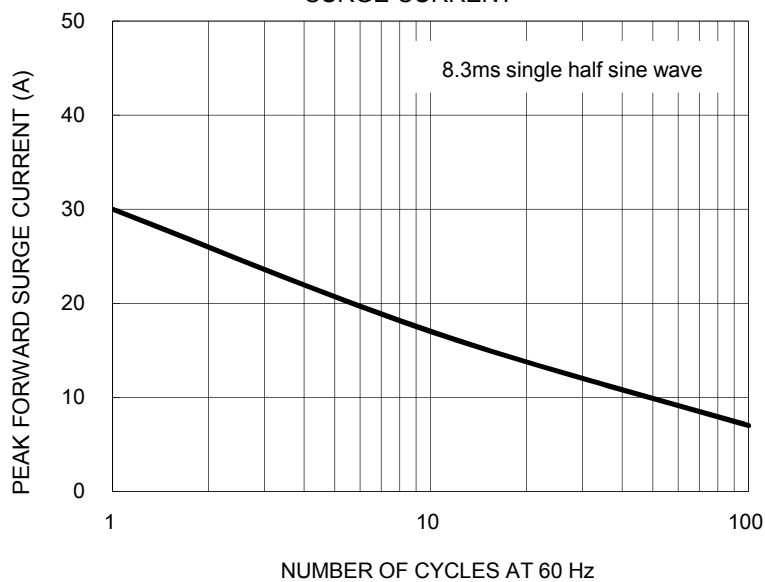
FIG. 3 MAXIMUM NON-REPETITIVE FORWARD SURGE CURRENT
