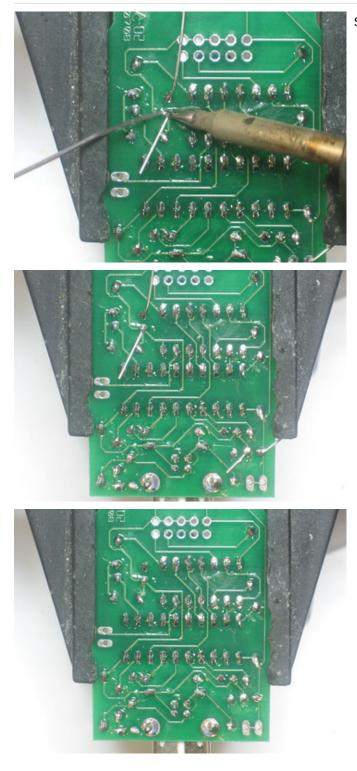
Solder and clip both capacitor's leads.
