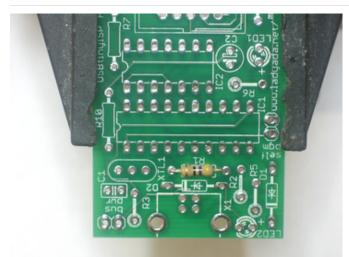
The first part to solder is a resistor, **R1**. This resistor has a 47ohm value, check the parts list to make sure you have the right one. Bend the two legs of the resistor so that its staple-shaped. Then slide the resistor into the PCB so that the outline matches the image on the silkscreen. Resistors are bi-directional so you don't have to worry about putting it in the wrong way.
