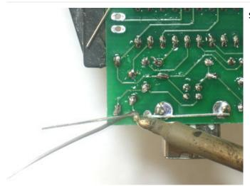
Solder and clip the two LEDs.
