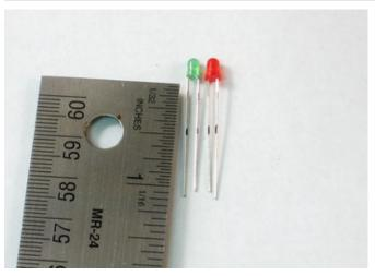
The two LEDs are next. They should stand-off a bit from the PCB so make a marking about 1/2" (1cm) from where the colored plastic ends.
