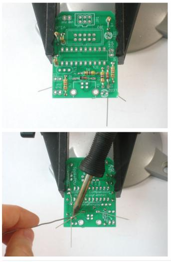
Next are the zener diodes. Diodes are directional so make sure to put them in as shown. There's a white stripe on the PCB drawing that matches the black stipe on the glass diode.
