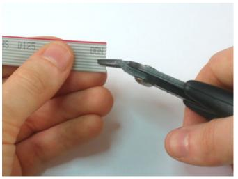
It's hard to find 6-conductor ribbon cable so you may end up with 10-conductor wire. (The kit ships with 6conductor) If so, just use your diagonal cutters (or a knife) to cut a notch so that the red stipe is on the 6conductor side.
