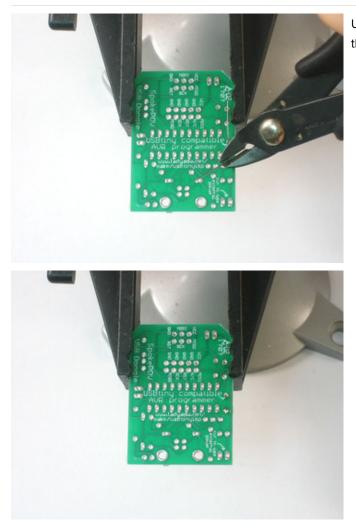
Use the diagonal cutters to clip the legs off just above the solder joint.
