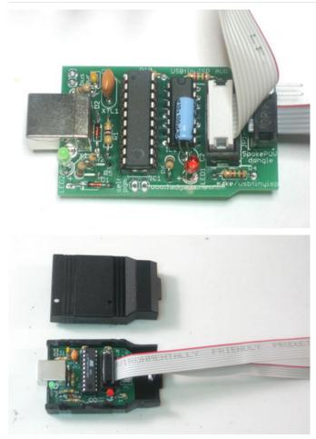
Plug in the two cables as shown, the red stripes on top and so that the cables don't bend over the plug (the case wont fit).
