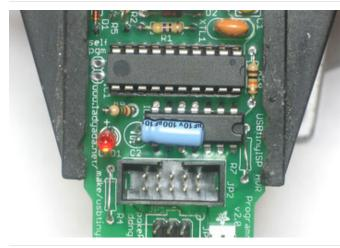
Finally, straighten the pins of the microcontroller and place it, so that the notch in the chip matches the notch in the socket (and the silkscreen) as shown.
