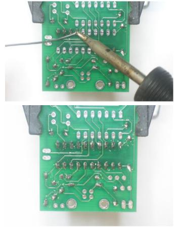
Tack two opposite corners of the socket, to keep it in place, and then solder all the pins.
