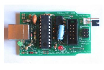
If you're not using the USBtiny to talk to a SpokePOV kit, and if you are using a target that has some load on the SCK and MOSI pins, you may need to replace R4 and R7 with jumpers as the 1.5K resistors will have trouble driving the load!
