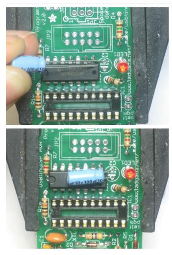
Next are the two capacitors, **C1** and **C2**. These provide some power supply filtering so that the USBtinyISP is less flakey. **C1** goes in the corner next to the USB connector. It is a non-polar ceramic capacitor so it can go in either way.
