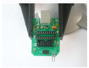
Next are the headers and the microcontroller socket. The 6-pin header has no direction so just put it in either way.
