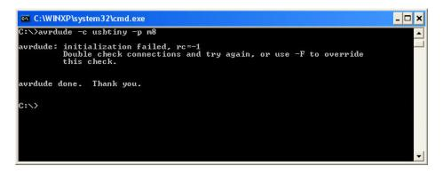
This response from avrdude means that it can talk to the programmer but the programmer can't talk to the chip.
