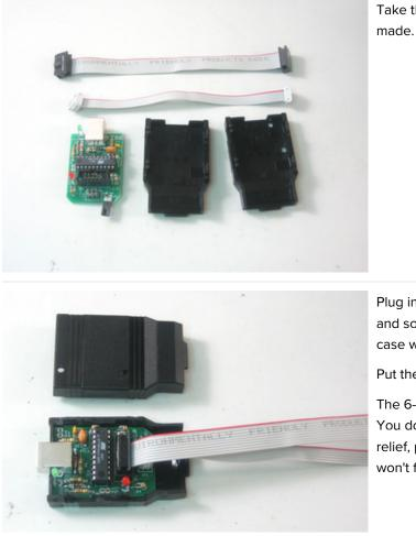
Take the PCB, two case halves and the cables you've made.
