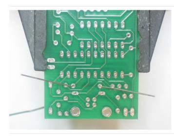
Bend the wire legs so that when the board is flipped over, it won't fall out.
