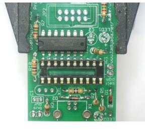
Next to be placed is the 74AHC125 buffer. This chip does a level-shifting conversion on signals from the USBtiny microcontroller to the device being programmed. This way you can safely program chips that vary from 1.8V to 5.5V voltage.
