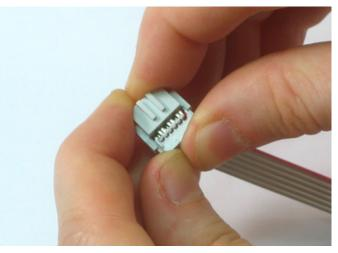
Get it started by just squeezing it with your fingers to make sure the wires are aligned properly. You won't be able to finish the cable this way so dont try!
