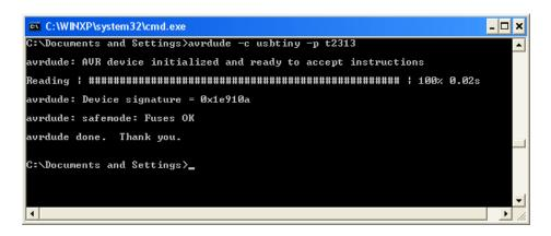
Using it is simple, just indicate usbtiny as the programmer type. The port option is ignored as it always uses USB.
