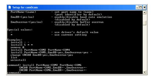
Type in **install PortName=COM2 PortName=COM6**, changing the COM2 to COM3 or COM4 if any of those are already being used. The second port should be anything between COM5 and COM10. Keep track of these ports because you'll need to refer to them later.
