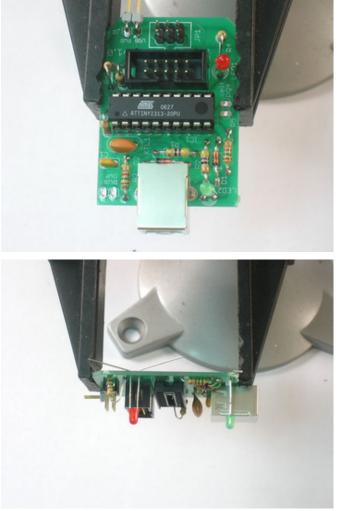
Place the LEDs as shown, the red one near the 10-pin header and the green one near the USB plug.
