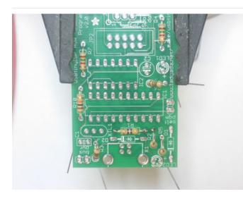
Now that you have a lot of practice with resistors, you can do the remaining 5 all at once. Place **R10** (10K pullup resistor), **R3, R5** and **R6** (1.5K resistors for the USB connection, LEDs and output buffer).
