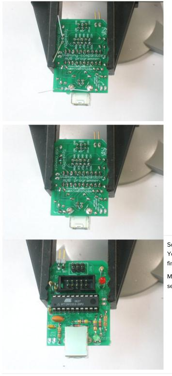
Soldering's done. Next up, insert the microcontroller. You can do this by gently bending the legs in using your fingertips or the tabletop.
