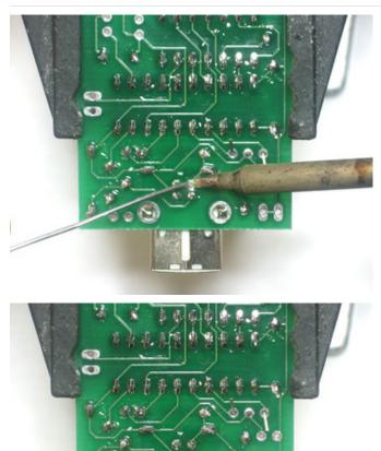
Solder in the three-pins of the oscillator and all 6 pins of the USB connector. Make sure to not bridge any of the square-pins and put plenty of solder on the mechanical tabs. These provide the resistance when you plug in a cable so it's important that they are soldered well, as shown here.
