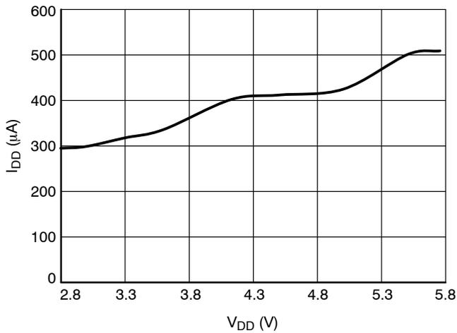
Figure 4. Supply Current vs.  $V_{DD}$
