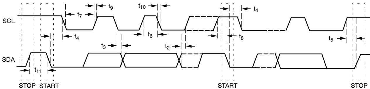
Figure 8. Serial Interface Timing
