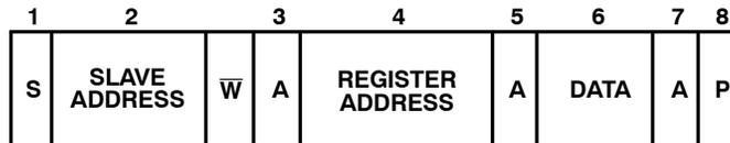
Figure 19. Write a Byte to a Register
