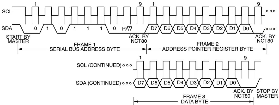
Figure 20. Writing a Byte to a Specified Address
