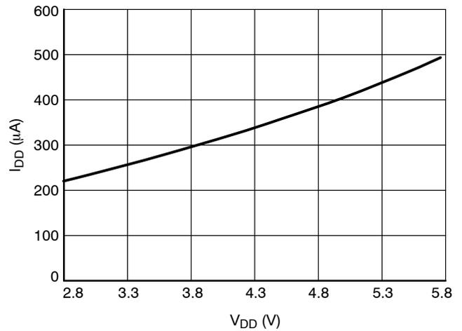
Figure 5. Shutdown Current vs.  $V_{DD}$
