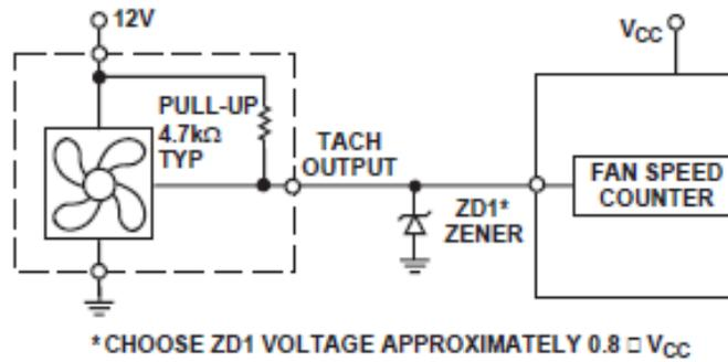
**Figure 11. Fan with Tach. Pull-Up to Voltage >6.5 V**
