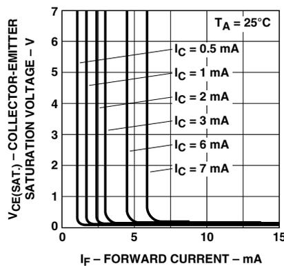
Figure 11. Collector-emitter saturation voltage vs. forward current.
