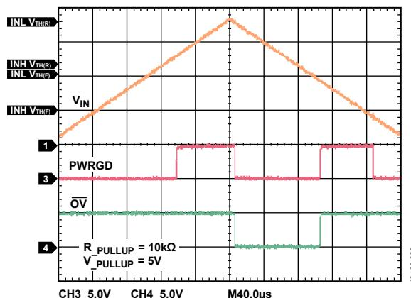
Figure 29. Propagation Delay
