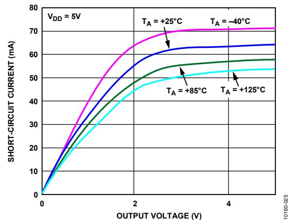
Figure 26. Output Short-Circuit Current vs. Output Voltage
