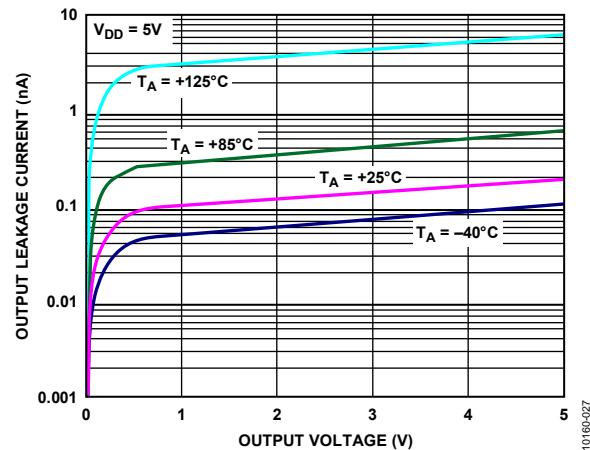
Figure 27. Output Leakage Current vs. Output Voltage
