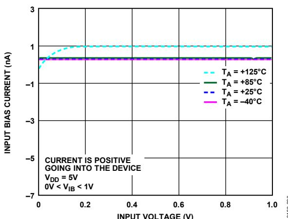
Figure 18. Low Level Input Bias Current vs. Input Voltage
