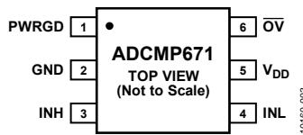
Figure 3. Pin Configuration
