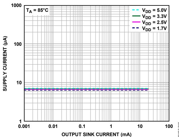
Figure 17. Supply Current vs. Output Sink Current for  $T_A = 85^\circ\text{C}$
