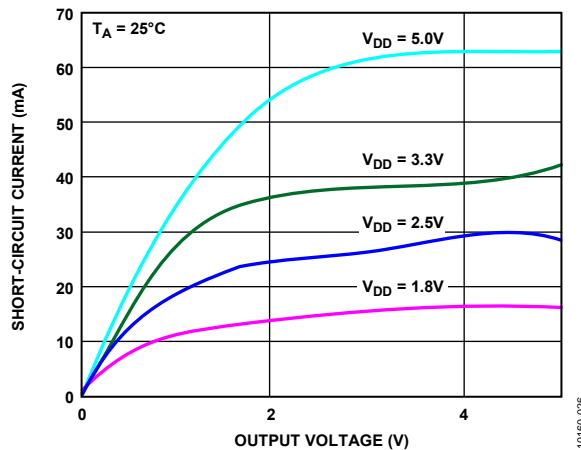
Figure 24. Output Short-Circuit Current vs. Output Voltage
