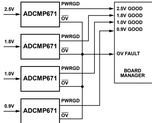
Figure 35. N Rails Monitoring with N + 1 Processor I/O
