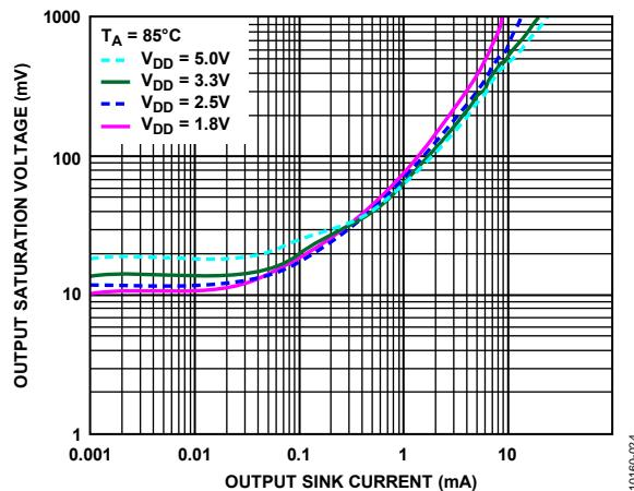
Figure 23. Output Saturation Voltage vs. Output Sink Current for  $T_A = 85^\circ\text{C}$
