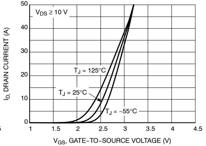
Figure 2. Transfer Characteristics
