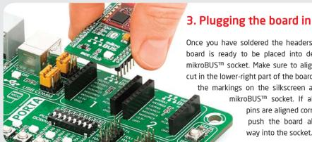
Once you have soldered the headers your board is ready to be placed into desired mikroBUS™ socket. Make sure to align the cut in the lower-right part of the board with the markings on the silkscreen at the mikroBUS™ socket. If all the pins are aligned correctly,
