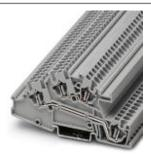
Installation level terminal block, Spring-cage connection, Cross section: 0.08 mm² - 4 mm², AWG: 28 - 12, Width: 5.2 mm, Color: gray, Mounting type: NS 35/7,5, NS 35/15
