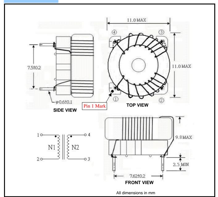
SPECIFICATIONSCommon Mode Choke TCK-053InductancePin 1-2: 830μH ±35%Pin 3-4: 830μH ±35%Test Condition: 100KHz/100mv<br/>Measurement Instrument: HP 4263B LCR MeterImpedanceDCR (Max): 31mΩ<br/>Measurement Instrument: HIOKI 3540 mΩ HITESTERRated CurrentIDC (Max): 3.3A<br/>Measurement Instrument: Agilent 34401A MeterRecommended Through Hole? 0.8 mm
