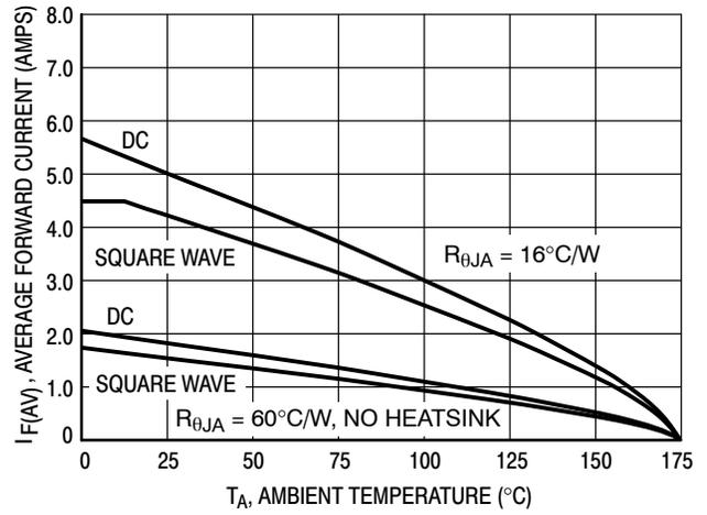
Figure 4. Forward Current Derating, Ambient, Per Leg
