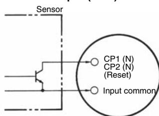
\*Operate with transistor ON
