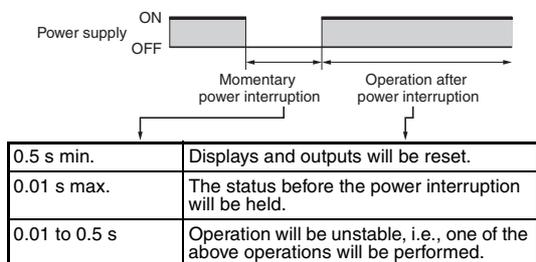
**Note:** Use a Counter with power failure backup memory (models ending with -M) if holding the status before the power failure is required when the power is interrupted.
