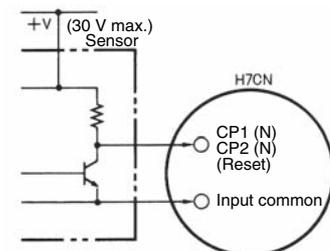
\*Operate with transistor ON
