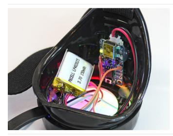
Power on the goggles by connecting the battery.
