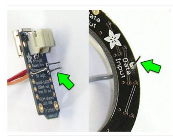
First, if you haven't already, clip off the tips of the soldered wires.
